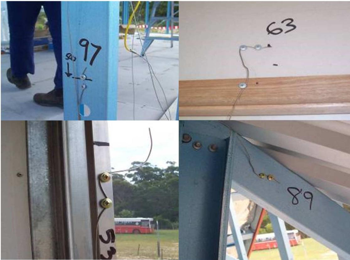
**Figure 5 Examples of thermocouples used for measuring surface temperatures (clockwise from top left: stud, plasterboard, roof truss, glass window)**
